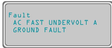
Figure 5-11. Ground fault error message
